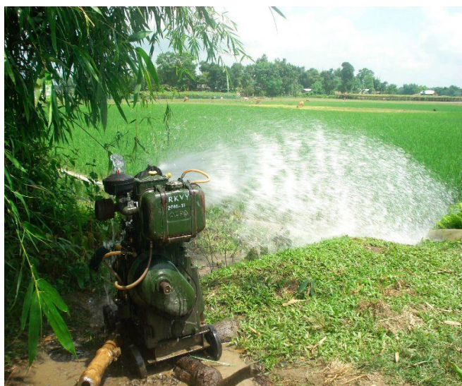
A Shallow Tube Well with diesel pump set supported under RKVY is being used to irrigate paddy in Nagoan District of Assam
