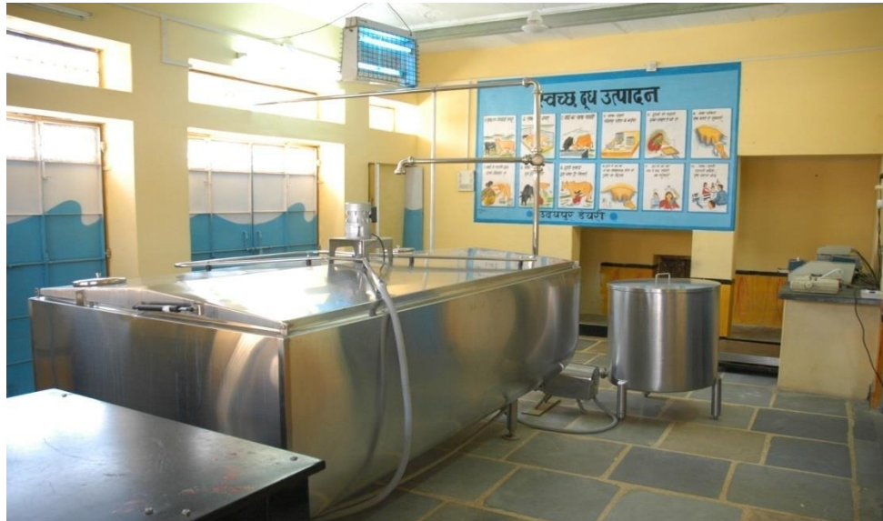
A Bulk Milk Cooler of 5000 litre capacity installed at a Dairy Cooperative Society in Rajasthan
